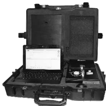
Measurement through transparent packages
